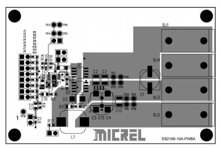
Figure 10. MIC2166 10A Evaluation Board Top Layer
