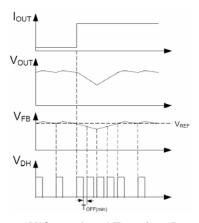
Figure 3. MIC2166 Load-Transient Response
