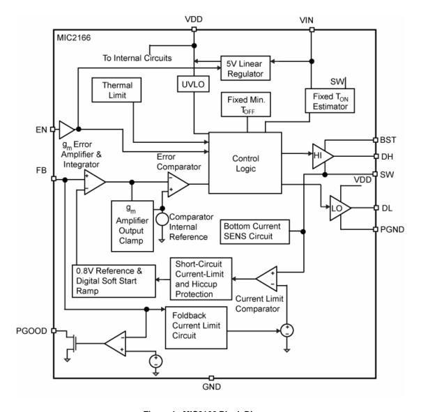
Figure 1. MIC2166 Block Diagram
