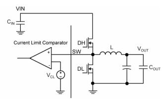
Figure 4. MIC2166 Current Limiting Circuit
