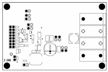
Figure 12. MIC2166 10A Evaluation Board Mid-Layer 1 (GND Plane)
