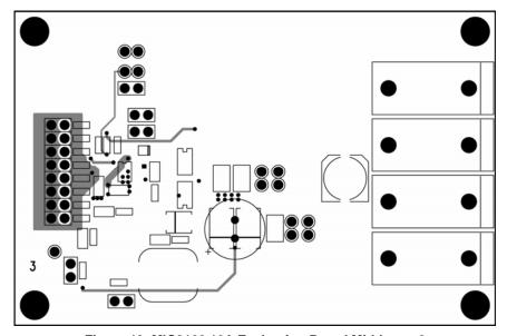
Figure 13. MIC2166 10A Evaluation Board Mid-Layer 2
