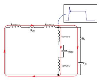
Figure 7. Snubber Circuit
