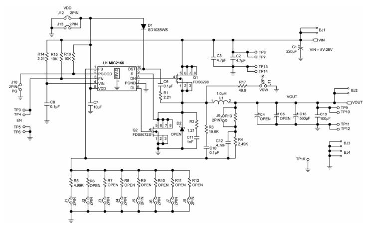
Figure 9. Schematic of MIC2166 8V-24V to 1.2V/10A Evaluation Board
