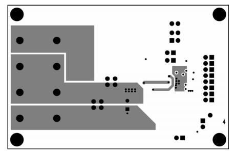
Figure 11. MIC2166 10A Evaluation Board Bottom Layer
