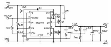
MIC2166 Adjustable Output 600kHz Buck Converter
