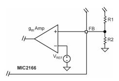
Figure 5. Voltage-Divider Configuration
